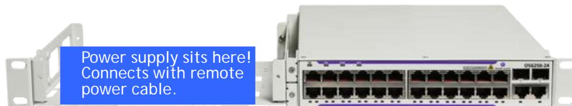
Customer may use the dual purpose mounting tray to mount a single unit in a 19" rack. The PoE supply secures to the side tray and may be connected to the switch unit using the supplied DB-15 remote connection cable.
