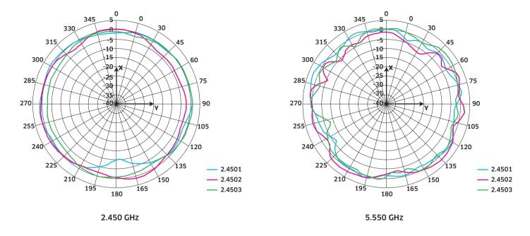
Figure 2. AP225 Antenna pattern plots: Elevation plane (side view)
